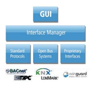
Connecting subsystems from building automation, security and communication systems via proprietary or standardised interfaces
